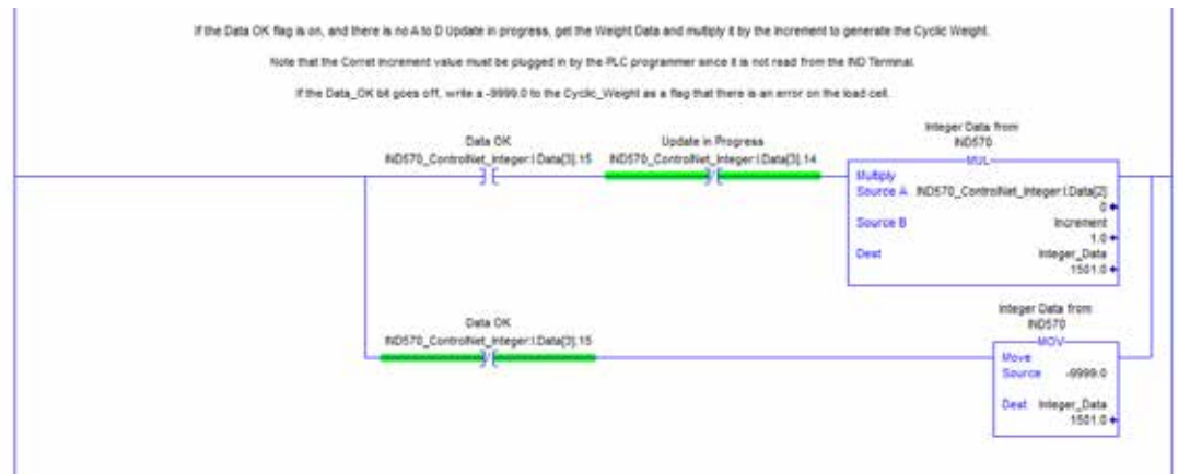
Figure 2-11: Filtering with Data_OK Bit and Two Data Integrity Bits, Integer or Division Mode
