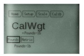
Figure 4-28: Calibration Weight Setup Screen
