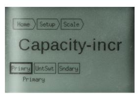
Figure 4-24: Capacity and Increment Setup Screen
