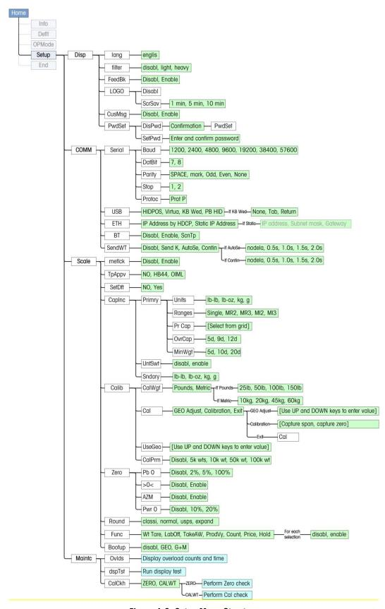
Figure 4-6: Setup Menu Structure
