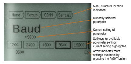
Figure 3-8: Typical Setup Screen
