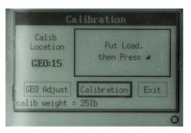
Figure 4-32: Calibration Sequence – Place Load
