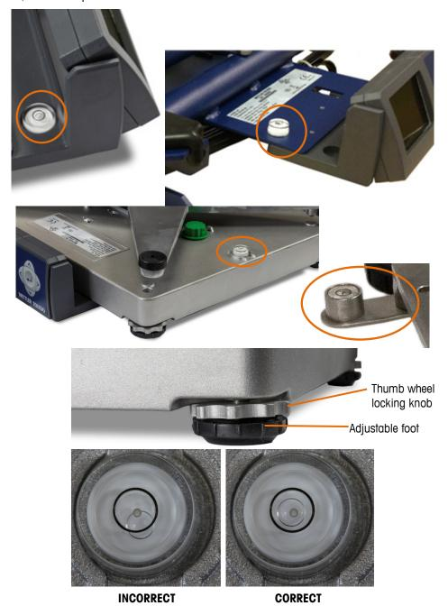
Figure 2-2: Leveling the Scale
