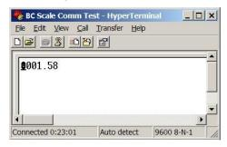
12. If the same weight is displayed on the scale and HyperTerminal screen, the scale is communicating correctly to the PC.
