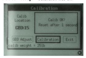
Figure 4-34: Calibration Sequence Successful
