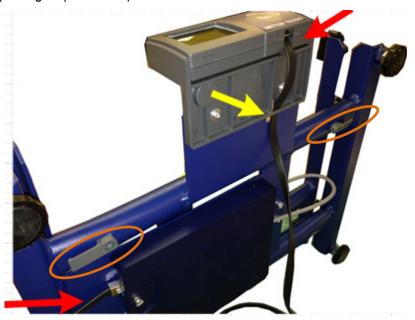
Figure 2-1: Display Installation
