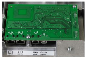
Figure 5-10: BC Scale PCB Mounting – Example
