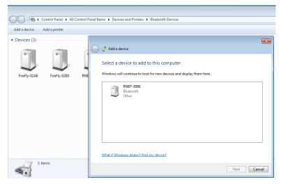
5. Select the device and click **Next**. The PC will try to establish connection with the BT device. If connection is established, the PC will create a pairing code. Click **Next**.
