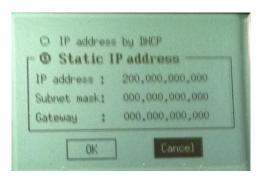
Figure 4-21: Ethernet Configuration Screen
