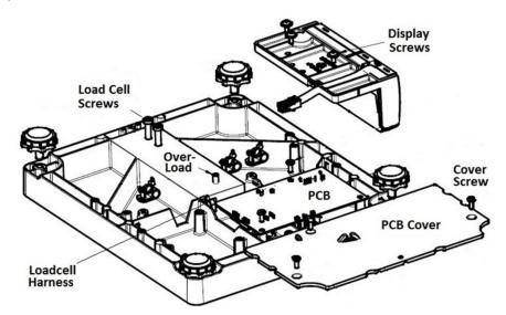
Figure 5-12: Bottom View of Scale
