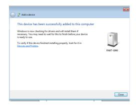
Connection is successful and the new device is added to the list of active devices with which the PC can communicate. The PC will install the driver of the BT device and create a virtual COM port.
