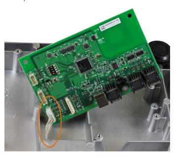
Figure 5-11: Load Cell Harness Connected to PCB
