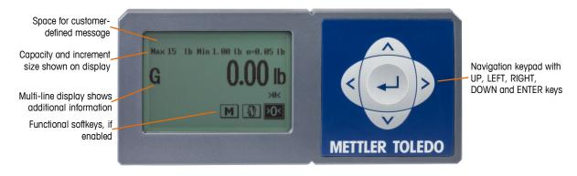
Figure 3-4: Weighing Mode Display
