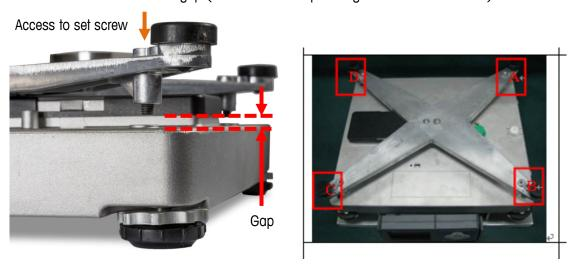
Figure 5-14: Location of Gap setting and designated scale corners
