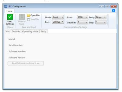
3. The BC Configuration Tool must be able to communicate with the scale. From the **Communication Settings** panel, select the proper parameters.
