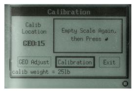
Figure 4-33: Calibration Sequence – Empty Scale Again
