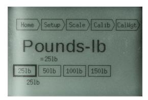
Figure 4-29: Calibration Weight Selection Screen, Pounds
