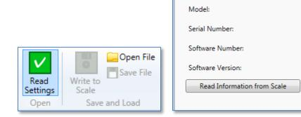
To read settings from the scale, either click the **Read Settings** button in the Ribbon control or click the **Read Information from Scale** button in the Info tab.
