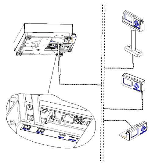
Figure 2-9: Second Display Installation
