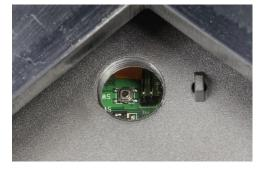
Figure 4-2: Access to Cal Button, BC30, BC3L, BC60, BC6L
