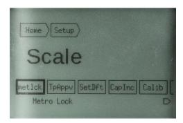
Figure 4-3: Scale Setup Menu
