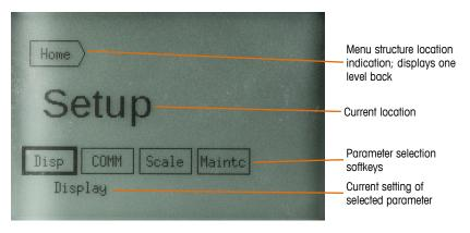
Figure 3-7: Initial Setup Mode Display
