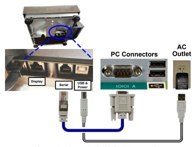
Power Supply required with RS232 connection
