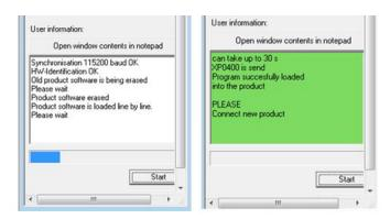
Figure 5-8: SimpleLoader Running (left) and Download Complete (right)
