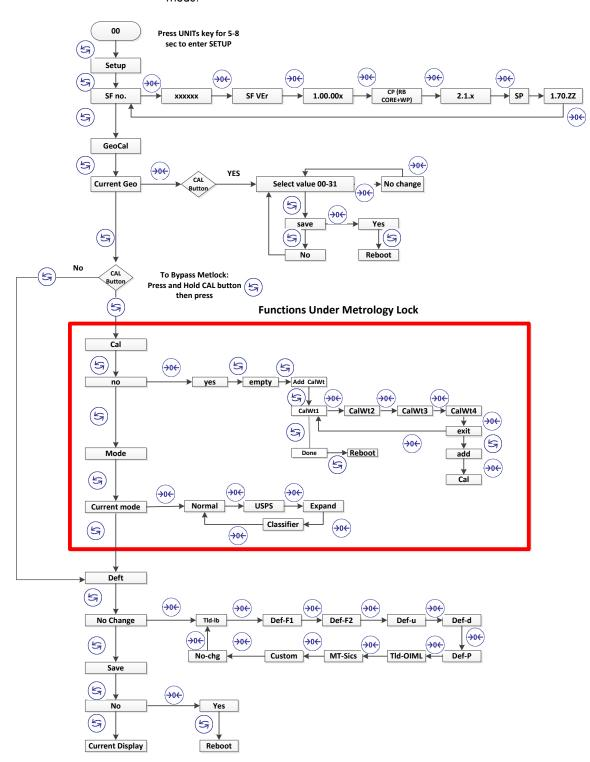
Figure 4-56: Parameter Configuration Using 7-Segment Display
