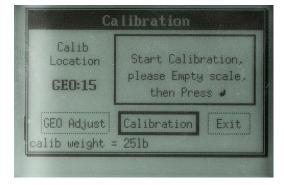
Figure 4-31: Start of Calibration Sequence
