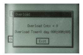
Figure 3-16: Maintenance – Overloads Display
