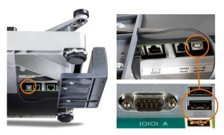
Figure 2-5: USB Connections, Scale and PC
