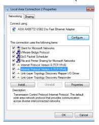
5. Open Properties. Enter the correct IP, Subnet Mask, and gateway address, then click OK.
