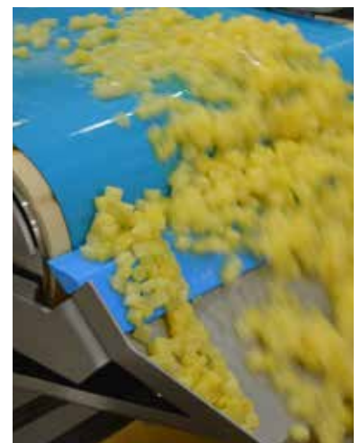
The wet characteristic of the pineapple makes it a challenging product for traditional metal detectors to inspect due to product effect, but Profile Advantage excels when inspecting these types of applications.
