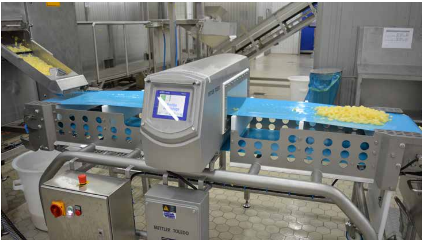
The Profile Advantage metal detector is combined with a conveyor system for easy integration into the production line.
