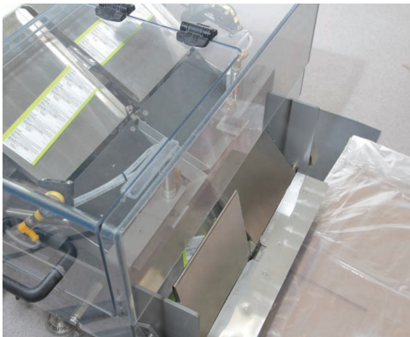
Packages slide down one of two chutes, stopping at a gate to be statically weighed with an extremely accurate electromagnetic force restoration (EMFR) weigh cell.
