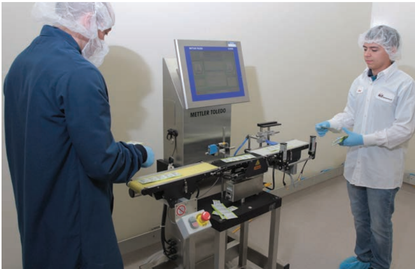
The XS1, designed to handle small, lightweight packages that are less than 200 g, is easy to use for offline hand feeding of product.
