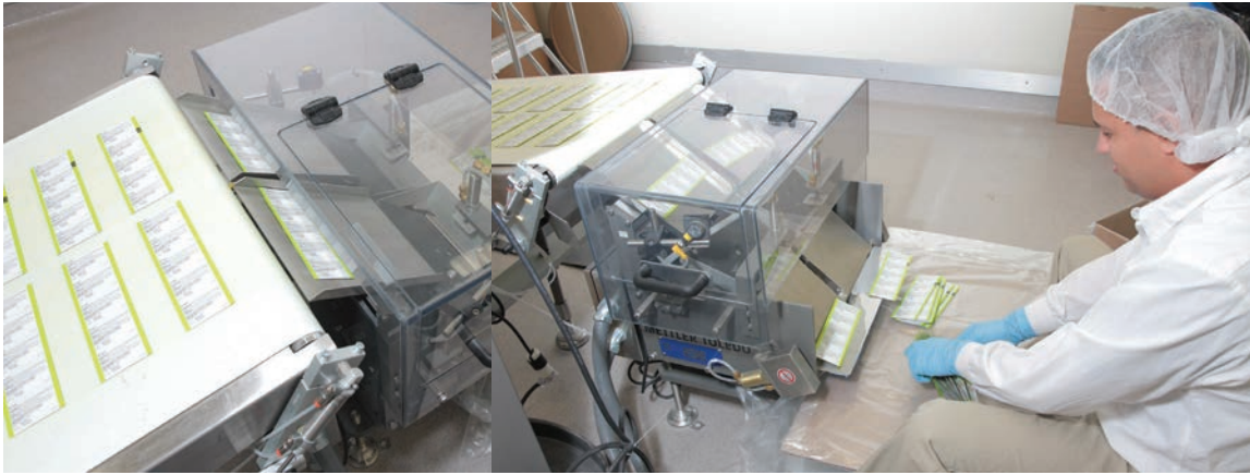
Inline weight inspection is less labor intensive and results in improved line efficiency while maintaining product quality.
