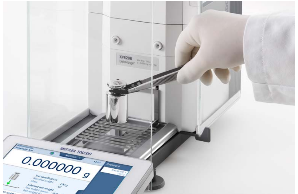
Correct weight handling with carbon-tipped tweezers.
