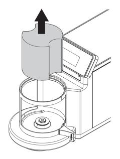
2 Open the weighing chamber door and remove the weighing pan from the weighing chamber.
