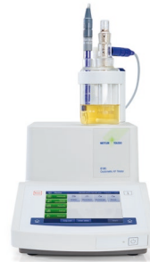
Water determination by Karl Fischer Titration
