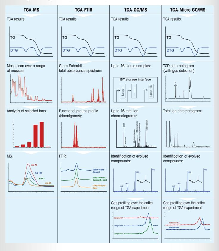
TGA-MS, TGA-FTIR, TGA-GC/MS and TGA-Micro GC/MS are powerful techniques that yield both quantitative (mass analysis, absorbance) and qualitative (identification, gas profiles) information.
