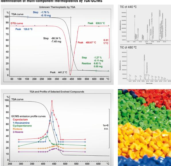
The identification of unknown materials is an important field in many R&D and QC areas. The following example illustrates how TGA-GC/MS can be applied for such a task. The TGA and DTG curves show that the sample starts to decompose at 300 °C with a 90% mass loss step (DTG peak maximum at about 440 °C and a shoulder peak at 480 °C).
