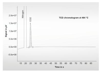
Coke is the residue formed after heating bituminous coal to high temperatures in the absence of air, and is typically used in the iron production process. Coke which is one almost pure form of carbon, evolves almost pure  $CO_2$  on burning. The quality of the coke can be determined by the amount of released  $CO_2$ .
